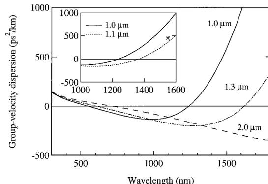
Fig. 1. Calculated GVD for 1.0-, 1.3-, and 2.0- $\mu\text{m}$ -diameter waist tapered fibers. The inset shows the GVD of the 1.0- and 1.1- $\mu\text{m}$  waist tapers in proximity to their second ZDWs, and the asterisk shows the dispersion value measured at 1550 nm.
