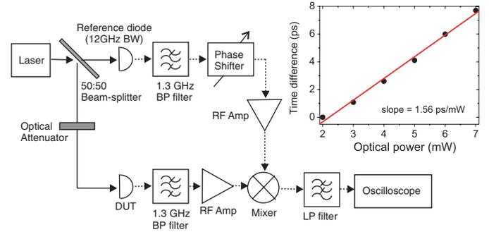
Fig. 4. Experimental setup for AM-to-PM conversion measurements of photodetectors.
