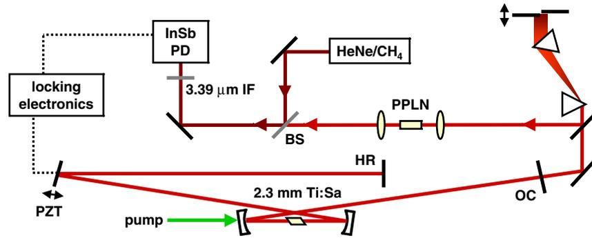
Fig. 7. Schematic of the DFG optical clock scheme [7].
