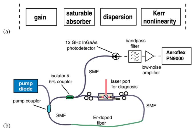
Fig. 2. (a) The four main effects governing pulse shaping in mode-locked lasers. (b) Schematic of the experimental setup: SMF, single-mode fiber.
