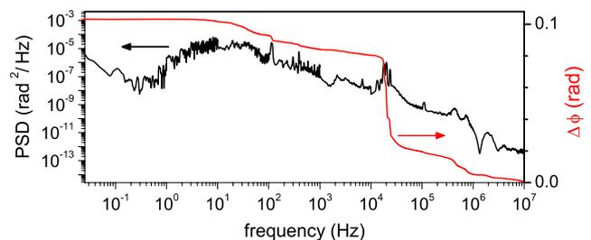
Fig. 6. Residual phase noise of the carrier-envelope phase [25].
