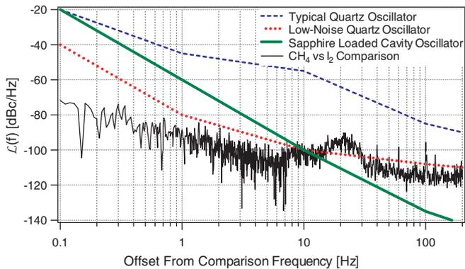
Fig. 8. SSB phase noise of the  $\text{CH}_4$  clock signal when compared to an iodine clock signal. Additional curves show the approximate single-sideband phase noise of extremely low-phase-noise microwave sources for comparison. All data were scaled to a 1-GHz carrier [7].
