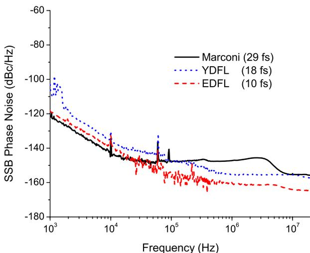
Fig. 3. Single-sideband phase noise of the YDFL (dotted line), EDFL (dashed line) and Marconi 2021 (solid line). The measurements are scaled to a carrier frequency of 1 GHz.
