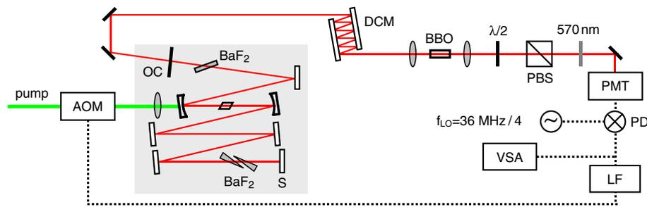
Fig. 5. Carrier-envelope phase stabilized 200 MHz octave-spanning Ti:sapphire laser. The femtosecond laser itself is indicated by the grey area. AOM, acousto-optical modulator; S, silver end mirror; OC, output coupling mirror; PBS, polarizing beam splitter cube; PMT, photomultiplier tube; PD, digital phase detector; LF, loop filter; VSA, vector signal analyzer. The carrier-envelope frequency is phase locked to 36 MHz [25].
