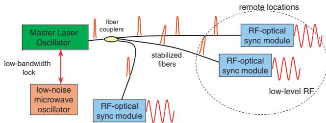
Fig. 1. Schematic of the optical timing synchronization system.
