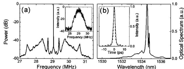
Fig. 2. Characteristics of the stabilized laser at 29 MHz. (a) rf spectrum in stabilized mode-locked and (inset) QSML operation. (b) Optical spectrum; inset, autocorrelation (solid curve) and autocorrelation of the zero-phase Fourier transform of the optical spectrum (dashed).
