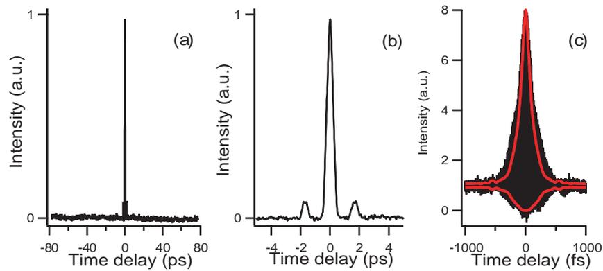
Fig. 3. Autocorrelation of the pulses from the Yb fiber laser, recorded over the indicated ranges of delay. (c) Measured interferometric autocorrelation (black) and envelopes calculated from the measured power spectrum (red).
