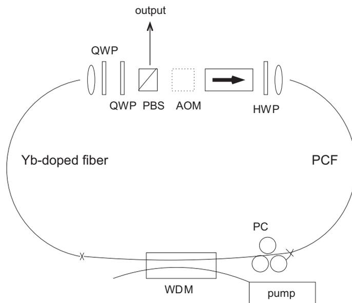
Fig. 1. Schematic of the laser. QWP: quarter-wave plate; HWP: half-wave plate; PBS: polarizing beam splitter; PC: polarization controller.
