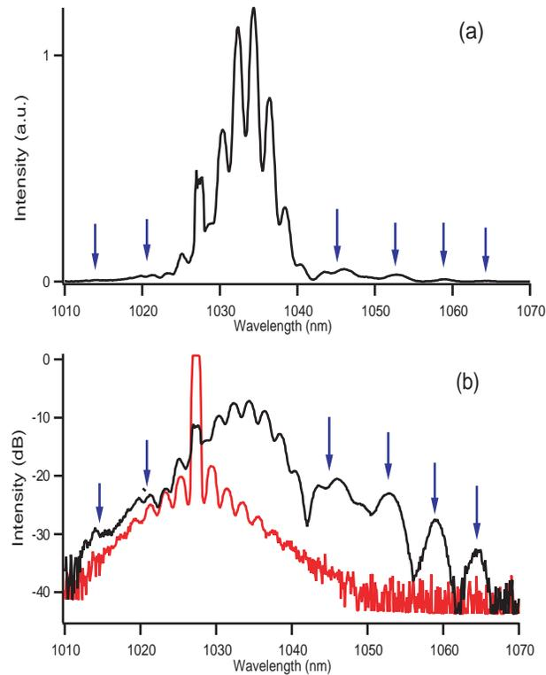
Fig. 4. Spectrum on (a) linear and (b) logarithmic scales. Spectral sidebands are marked with arrows. The cw lasing spectrum of the laser (red line in (b)) is also shown for comparison.
