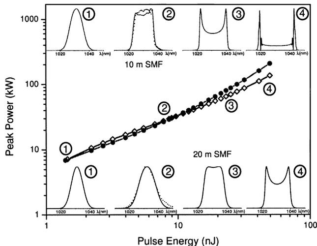
Fig. 2. Peak power of amplified and dechirped pulses as a function of pulse energy with stretching in 10 m (filled symbols) and 20 m (open symbols) of SMF. Insets: Calculated pulse spectra (1), (2), (3), and (4) are for pulse energies of 1.4, 8, 25, and 50 nJ, respectively. Note the agreement of calculated spectra with experimental results for 8-nJ pulse energy.
