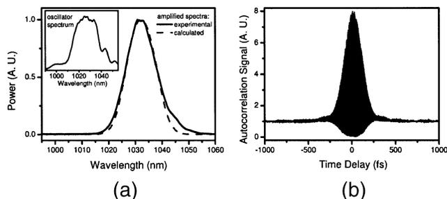
Fig. 3. (a) Experimental and calculated spectra of the amplified pulses. Inset: Spectrum of the pulses from the oscillator. (b) Interferometric autocorrelation of the dechirped pulses.
