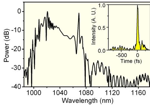
Fig. 1. Results of numerical simulations of the Yb fiber laser. Main figure: power spectrum plotted on logarithmic scale. Inset: temporal intensity profile of dechirped output pulse.
