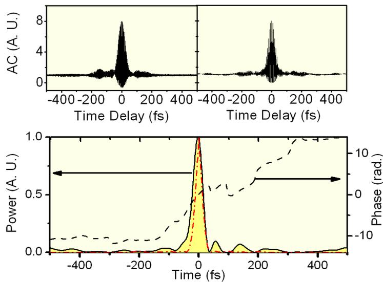
Fig. 3. Output of the Yb fiber laser. Measured interferometric autocorrelation (top left panel) along with the interferometric autocorrelation of the pulse retrieved by PICASO (top right panel). Bottom panel: retrieved intensity and phase profiles compared to the transform-limited pulse (dash-dotted line).
