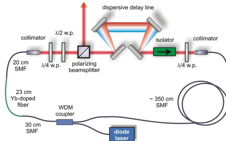
Fig. 2. Schematic of the Yb fiber laser. w.p.: waveplate.
