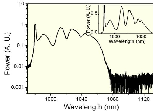
Fig. 4. Measured power spectrum plotted on semi-logarithmic scales. The component at 980 nm is unabsorbed pump light. The inset shows the spectrum on linear scales.
