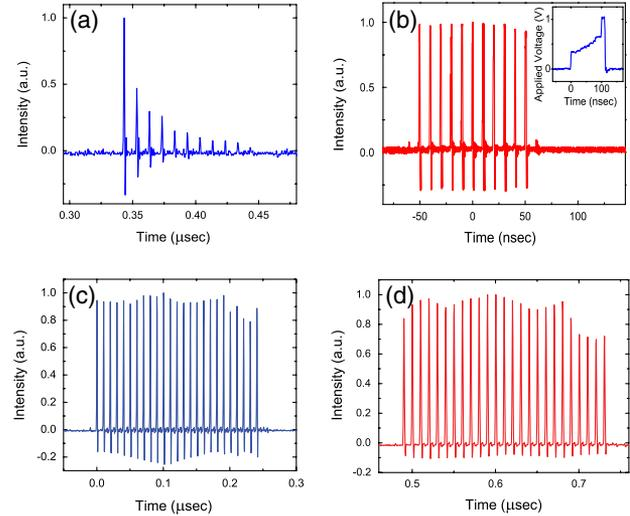
Fig. 2. (Color online) Temporal profile of the amplified burst with total energy of (a) 150  $\mu\text{J}$ , with no precompensation; (b) 660  $\mu\text{J}$ , comprised of 11 60  $\mu\text{J}$  pulses (pulse-energy variation of <2%); (c) 775  $\mu\text{J}$ , comprised of 25 31  $\mu\text{J}$  pulses (pulse-energy variation of <5%); and (d) 1 mJ, comprised of 25 40  $\mu\text{J}$  pulses (pulse-energy variation of <7%). Inset to (b), corresponding AOM gate signal.
