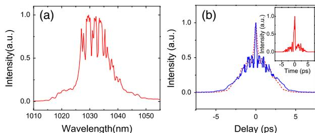
Fig. 3. (Color online) (a) Measured optical spectrum of the burst-mode amplifier output with  $40 \mu\text{J}$  energy per pulse and total of  $1 \text{ mJ}$  energy per burst. (b) Measured (blue solid curve) and retrieved (red dashed curve) autocorrelation of the de-chirped pulses at the same energy level. Inset: retrieved pulse shape using the PICASO algorithm based on the autocorrelation and spectrum measurements.
